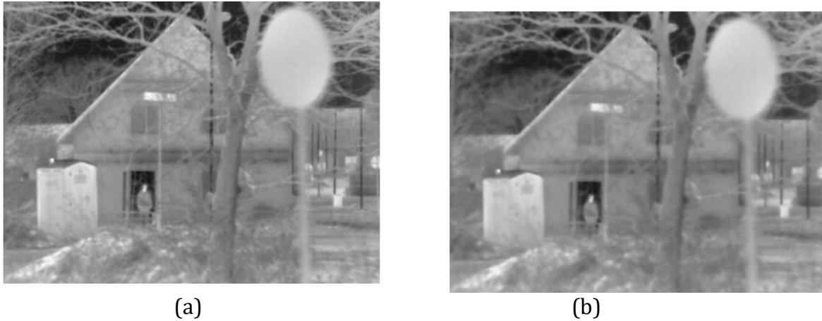
Figure 2.1 (a)The infrared image.(b)the guided filter image
