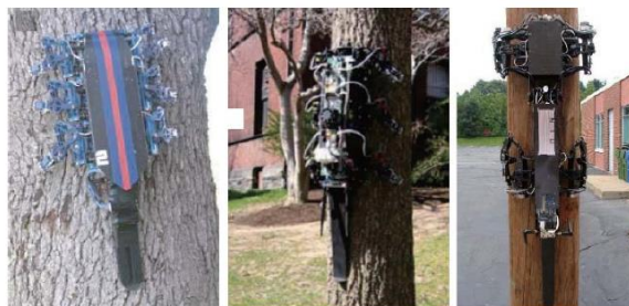
Fig.3 Multi-foot climbing robot
