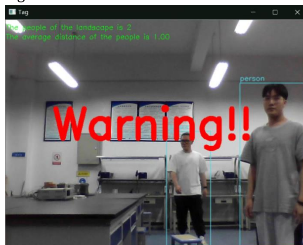
Figure 9: Human flow detection of PC software
